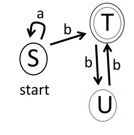
With string "abab" we start in state S, stay in S on input 'a', go to state T on input 'b' and then have nowhere to go on input 'a'. Again, we do not accept the string. The only strings accepted are those for which the automaton consumes all of the letters in getting to an accept state.
