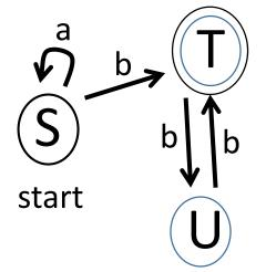
Here you see labeled circles that are *states*, and labeled arrows that are *transitions*. One of the states is marked "start". One of the states has a double circle; this is a *terminal state* or *accept state*.
